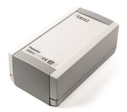
The AMB8627-M-RP2 is a battery powered unidirectional repeater according to the EN 13757 Wireless M-BUS standard. It is suitable for environments needing range extension in order to reduce the amount of Smart Meter Gateways in the meter reading network. Repeating of OMS frames is supported.
